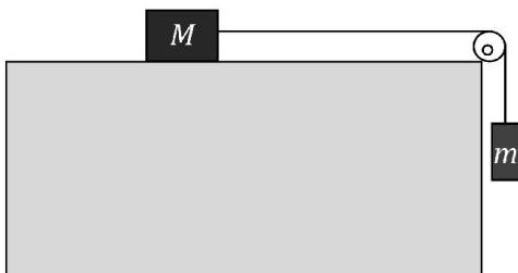
$$\left. \begin{array}{l} M_{\text{جسم}} : T - f = Ma \\ m_{\text{جسم}} : mg - T = ma \end{array} \right\} a = \frac{mg - f}{M + m}$$
