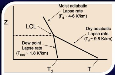
To find LCL graphically on tephigram or skew-T diagram, draw lines upward from the surface temperature and surface dewpoint along the dry adiabat and mixing ratio, respectively. They intersect at the LCL. This determines the cloud base.
