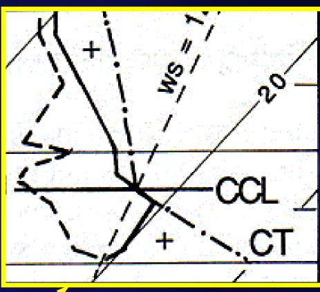
CCL - Convective Condensation Level - is found by following surface  $w_s$  up to ambient temperature profile. It is the LCL for a parcel reaching the CT.
