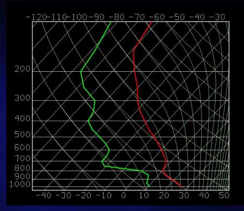
The area between 700 and 800mb is an example of an absolutely stable layer.
