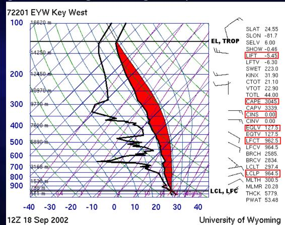
This is a very unstable sounding. A large CAPE can be inferred from the large area of red shading between parcel and ambient temperature profiles. Note that CAPE greater than 3000 J/kg indicates the probability of severe convection. Indeed, hurricane Isadore was not far from Florida at the time of the sounding. The LCL and LFC are at the same level in his sounding. The tropopause and EL also coincide.
