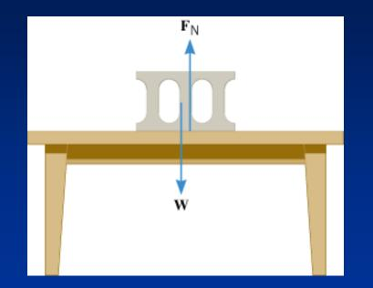
The normal force  $F_N$  is one component of the force that a surface exerts on an object with which it is in contact, namely, the component that is perpendicular to the surface.
