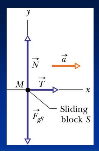
$a_x$  must also equal |a| as the rope is under tension (and we assume doesn't stretch)
