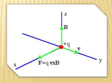
What happens if the velocity is not perpendicular to the field? In this case, we can resolve the velocity into two components, one parallel to the field and one perpendicular.
