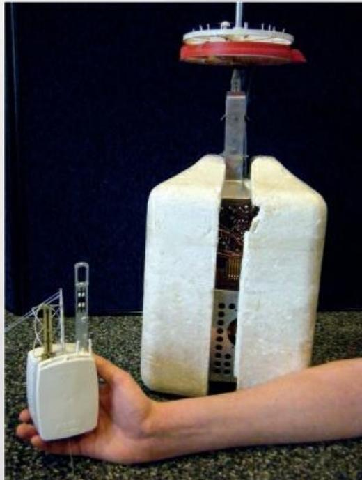
A radiosonde launch. The assembly consists of a radiosonde (the small white box at the bottom), a parachute (the red piece of plastic) and a helium balloon, which usually measures about 2 m across at launch.
