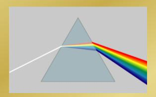
In optics, *dispersion* is a phenomenon that causes the separation of a wave into spectral components with different frequencies, due to a dependence of the wave's speed on its frequency. If velocity of propagation is independent of freq i.e. that is there is no dispersion then all component of the pulse travel with same velocity so the velocity of the resultant is the same as the phase velocity.
