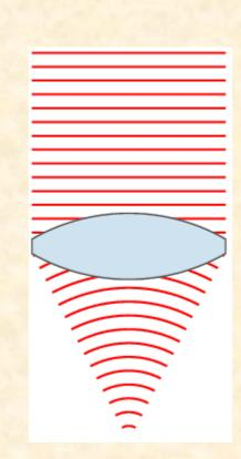
Here, plane wavefronts become spherical after going through the lens.
