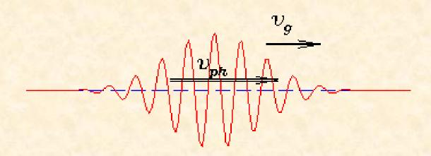
Figure: A WAVE PACKET moving at  $v_{\rm g}$  with ``wavelets'' moving through it at  $v_{\rm ph}$ .
