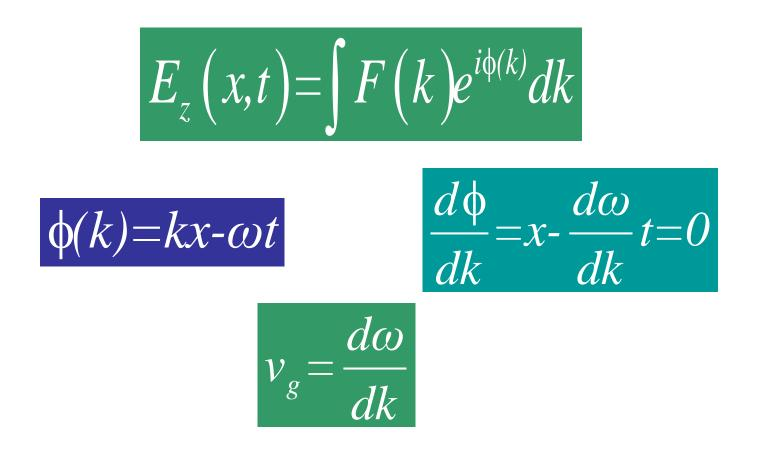
The upshot of the above discussion is that information (*i.e.*, an individual wave-pulse) travels through a dispersive media at the group velocity, rather than the phase velocity. Hence, relativity demands that the group velocity, rather than the phase velocity, must always be less than .
