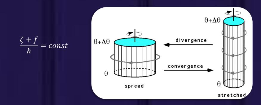
The vortex of air on the left in is broad and slow. When the air converges, the column stretches, i.e. h increases. To maintain potential vorticity, the air spins faster ( $\xi$  increases), resulting in the streched vortex on the right. Divergence, on the other hand, causes vortex spreading and slows down the rate of spin.
