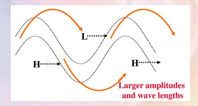
Relation between stream lines and trajectories in a retrogressive flow
