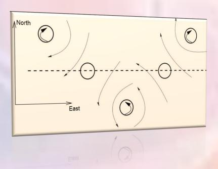
This perturbation vorticity field will induce a meridional velocity field, which advects the chain of fluid parcels southward west of the vorticity maximum and northward west of the vorticity minimum, as indicated in Fig.
