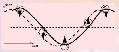
Perturbation vorticity field and induced velocity field (dashed arrows) for a meridionally displaced chain of fluid parcels.
