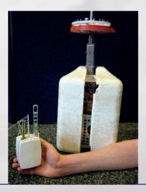
A radiosonde launch. The assembly consists of a radiosonde (the small white box at the bottom), a parachute (the red piece of plastic) and a helium balloon, which usually measures about 2 m across at launch.
