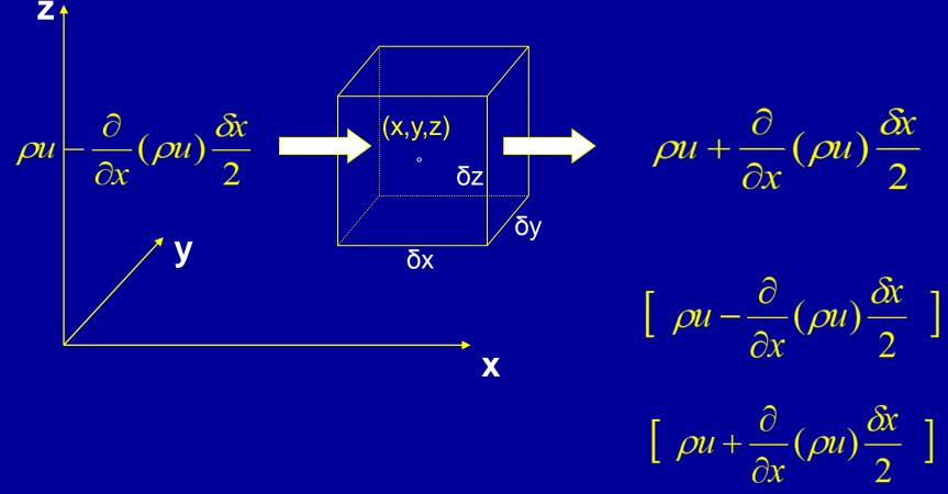
Since the area of these faces is  $\delta y \, \delta z$ , the net rate of flow into the volume owing to the x velocity component is:
