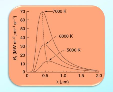
Blackbody radiation curves at three different temperatures (K; see legend in upper right corner)
