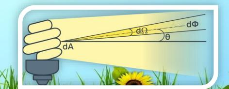
The spectral radiance can be visualised in terms of the photons emerging from a small area  $\Delta A$  with unit normal s, centred at a point r
